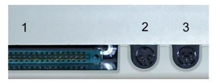
Some FE3 cartridges have an integral lead with a plug, others have two sockets. Either
